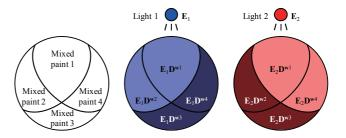
Figure 3. Metamerism of four sets of mixed paint illuminated by two different lights.
