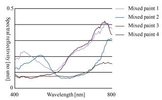
Figure 7. Spectral reflectance of four mixed paints.
